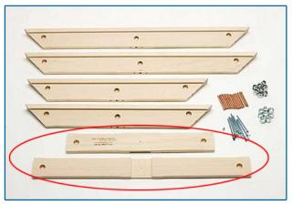
1. Assemble braces first. (Circled in red above.) Lay braces with the holes face up; the alphanumeric markings should be on the perimeter of the braces, the markings should be alphabetical, clockwise. Attach braces via the pre-drilled holes at each intersection with the screws provided. (As shown above, two braces will have just one intersection.)
